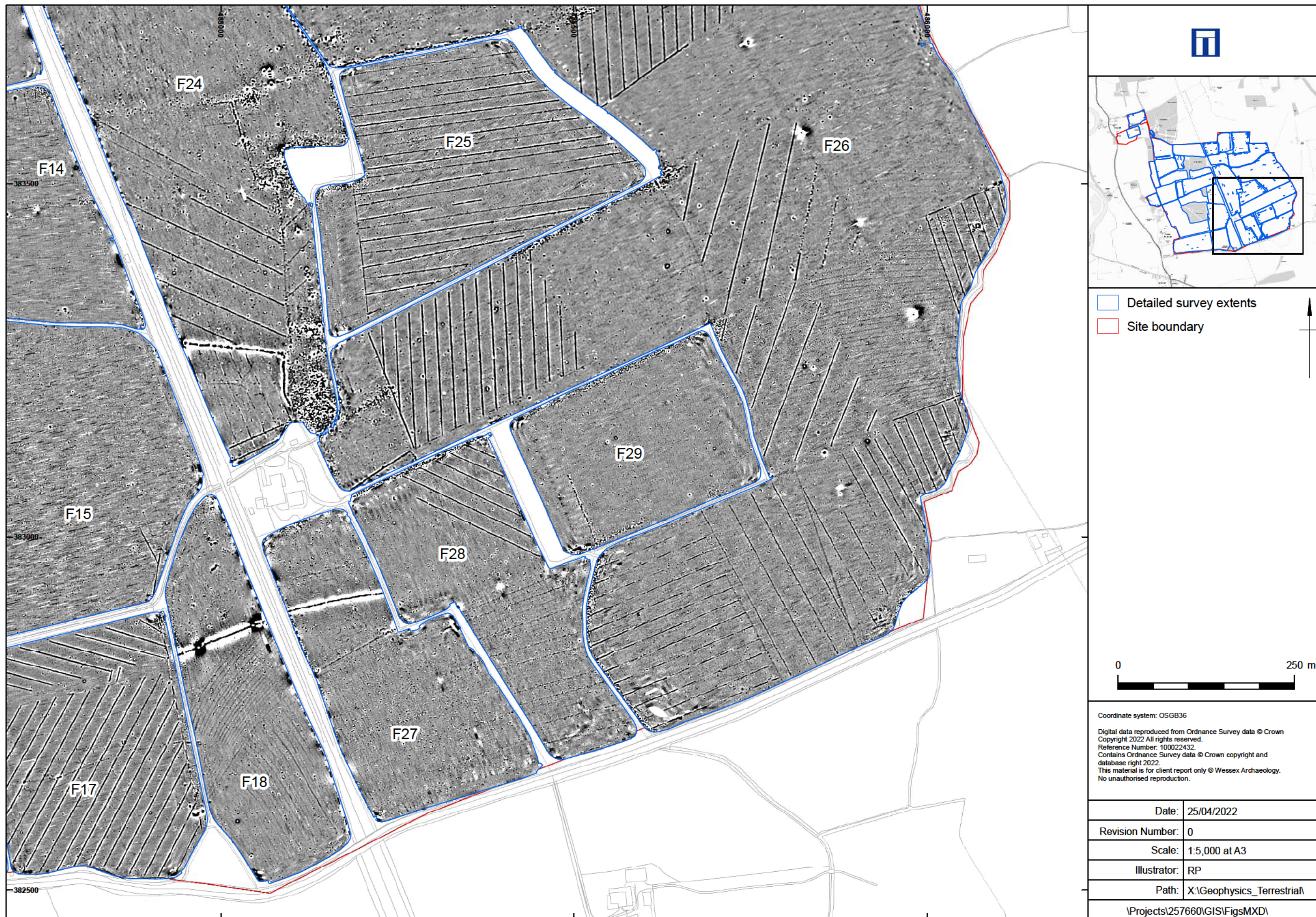
Detailed gradiometer survey results: greyscale plot (Fields 24 - 29)
